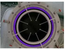
The bezel chuck in action facilitates coaxial assemblies for large components (10in X 20in) saves > \$10K in development cost
