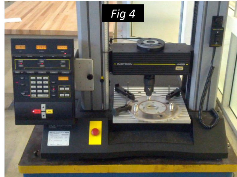
Bond tensile testing using FM!000 epoxy
