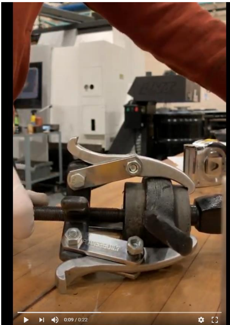
Control arm bushing replacement
